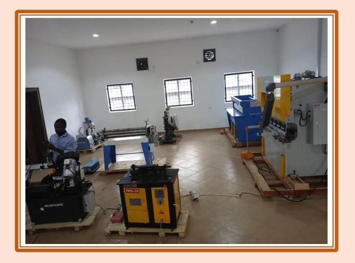
MACHINE TOOL WORKSHOP WITH A 3D PRINTER, A HYDRAULIC PRESS BRAKES, SWING BEAM SHEARS, AN IRONWORKER, PLATE ROLLS, PROFILE ROLLS, HORIZONTAL BAND SAWS, A WELDING MACHINE AND A LATHE MACHINE
