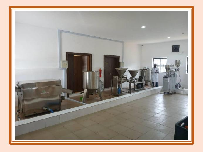
TOMATO PASTE PRODUCTION LINE WITH A TOMATO BUBBLE WASHING MACHINE, A PREHEATING POT, A TOMATO MILLING MACHINE, A TOMATO SMOOTH CRUSHING MACHINE, A TOMATO MIXING AND BOILING TANK, A VISCOUS TRANSFER PUMP AND INDUSTRIAL HOSE AND A PASTE SACHETS PACKAGING MACHINE
